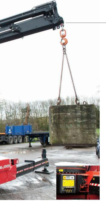
crane are compatible; checking that equipment such as AdBlue and fuel tanks, exhaust systems, etc, will have been repositioned where necessary; specifying the right PTO (power takeoff), in terms of flow, pressure and usage, if factory fitted; and agreeing appropriate electronic controls, such as PTO and parking brake interlocking, engine stop-start and speed-up, and suspension lock out.
