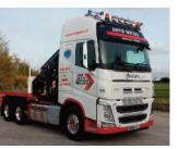
Above and right: David Watson Transport approached Fassi dealer **Walker Crane Services to** install the largest crane possible on a three-axle tractor unit - for heavy lifting on sites with limited space. Walker collaborated with Volvo, specifying a 10-tonne front axle capable of hosting Fassi's newest F820RA.2.26 - an 82 tonne-metre crane with six hydraulic extensions while not compromising the truck gvw
